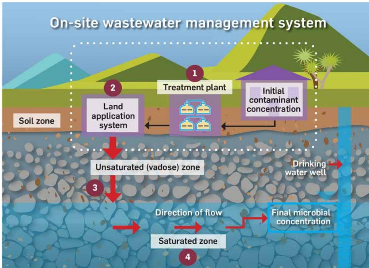
**Fig. 7.** / This diagram shows the opportunities for microbial and chemical removal in an on-site wastewater management system and the receiving environment: 1) the OWMS treatment plant, 2) land application system, 3) vadose zone (unsaturated zone) and 4) saturated zone.
