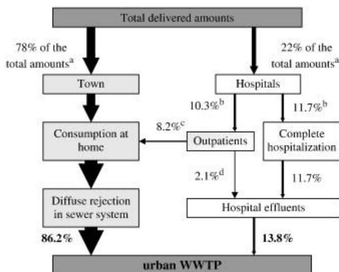
**Figure 2 Theoretical input pathways for anticancer drugs to the aquatic environment**
