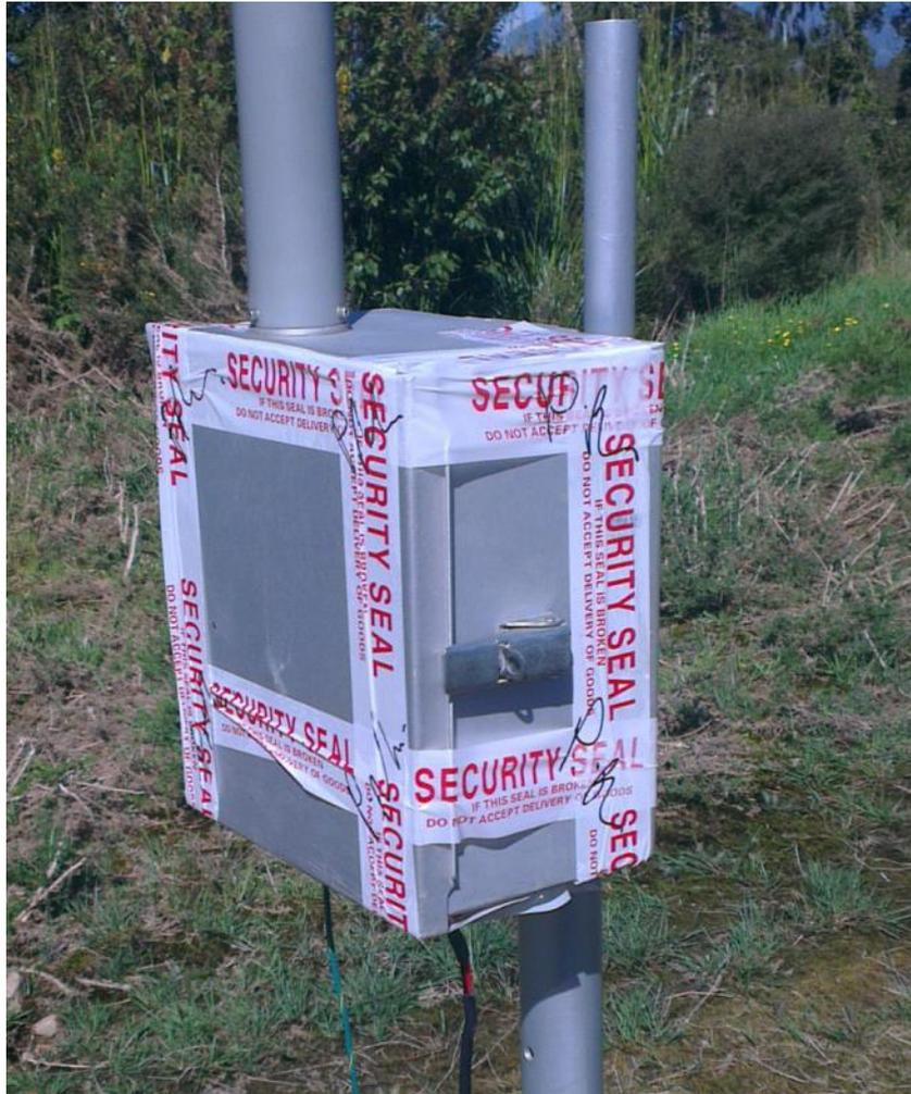
**Photo 1** Photograph of the monitoring station at site Z-4 illustrating the security tape on the device with signatures of the field technicians across all joins. The sample filter is situated inside the metal case.
