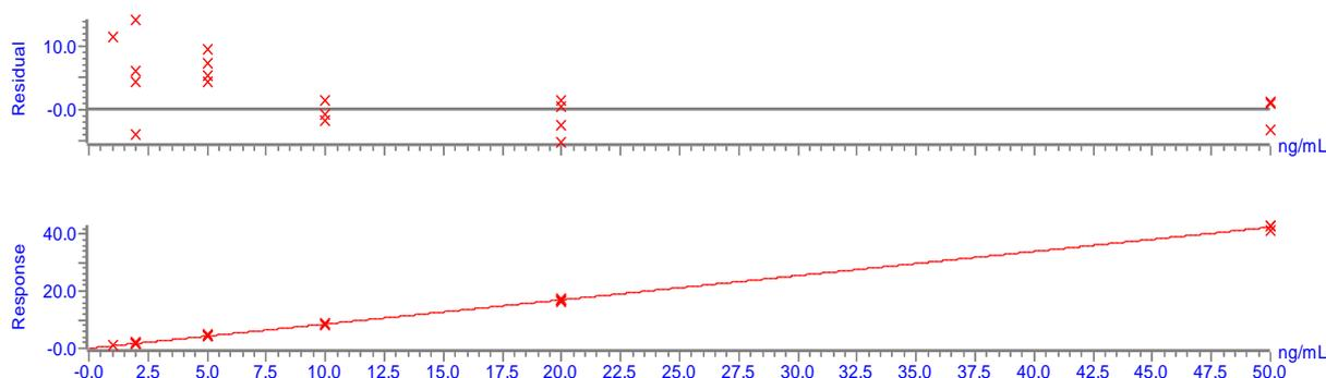
Figure 7. Typical calibration curve for  $\beta$ -N-methylaminoalanine (BMAA) using  $^{13}\text{C}^{15}\text{N}_2$ -BMAA as an internal standard, showing linear working range of 1–50 ng/mL.
