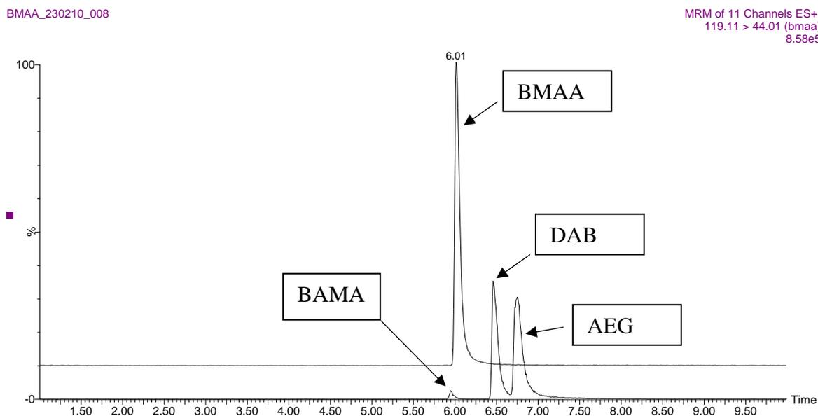
Figure 5. LC-MS/MS chromatograms for the  $\beta$ -N-methylaminoalanine (BMAA) quantitation transition ( $m/z$  119.1>44), where BMAA was analysed (top chromatogram) and BMAA isomers analysed (bottom chromatogram) –  $\beta$ -amino-N-methylalanine (BAMA), diaminobutyric acid (DAB) and N-(2-aminoethyl)-glycine (AEG).
