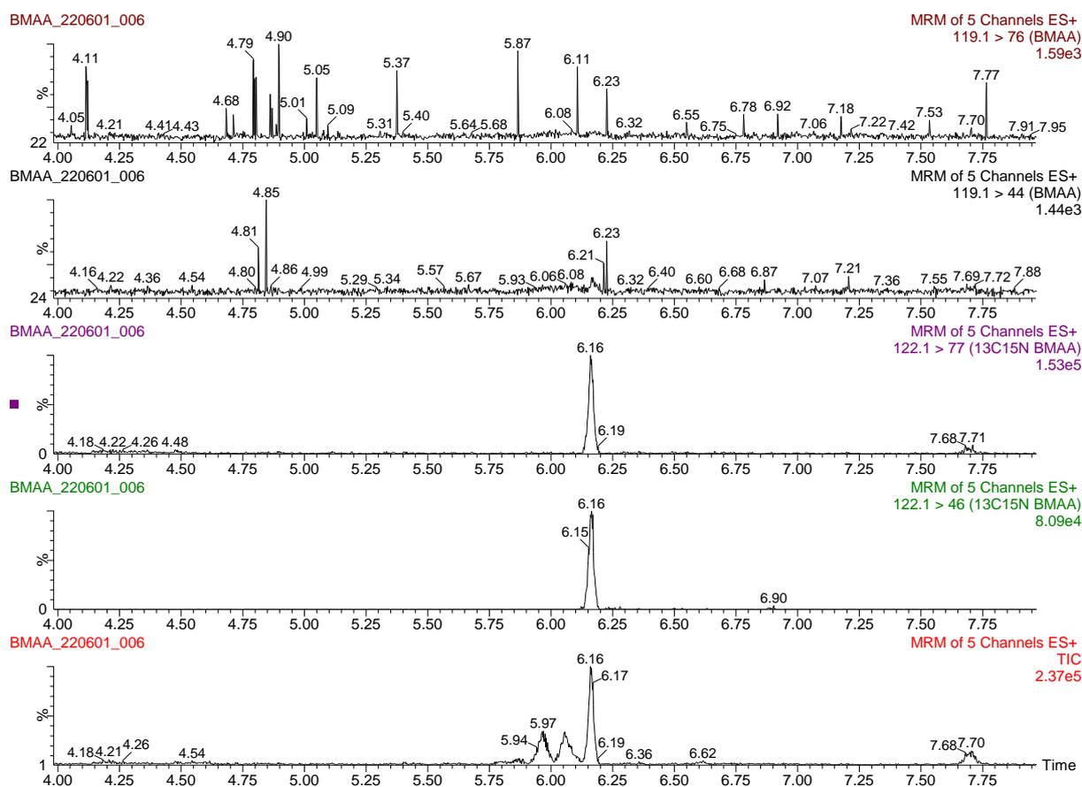
Figure 6. LC-MS/MS chromatograms for a hydrolysate of the ALG-06 sample spiked with 10 ng/mL of  $^{13}\text{C}^{15}\text{N}_2$ - $\beta$ -N-methylaminoalanine (BMAA). From top to bottom: quantitation and confirmation BMAA transitions, two transitions for  $^{13}\text{C}^{15}\text{N}_2$ -BMAA, and total ion chromatogram for all transitions.
