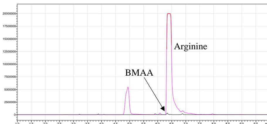
Figure 3. LC-MS/MS chromatograms showing  $\beta$ -N-methylaminoalanine (BMAA) and arginine before solid-phase extraction clean-up.
